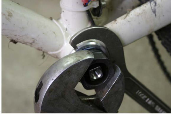
Fig.9 Hold cup while lock ring is tightened.
