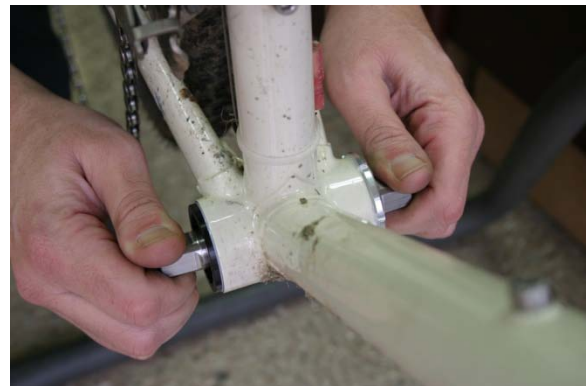
Fig.11 Checking for play.
