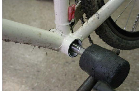
Fig.6 Gently tapping spindle into place.
