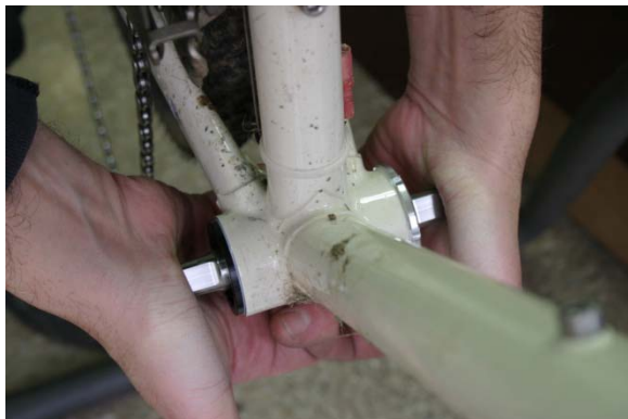
Fig.10 Checking for lateral play.
