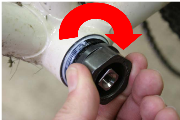
Fig.7 Tighten non-drive side cup, clockwise.
