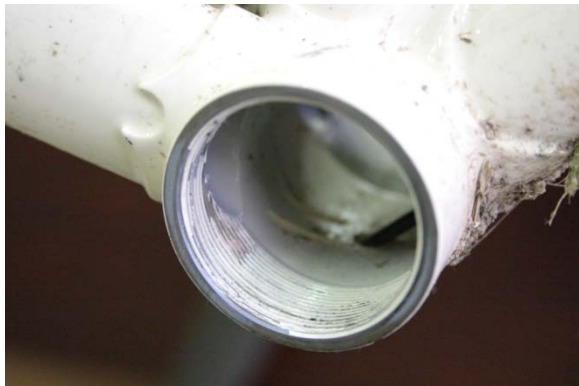
Fig.1 BB threads clean and ready for install.
